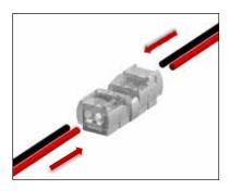
1. Cut the wire to the required length, insert it into the corresponding hole and slot of the connector, and insert it to the end (note: the parallel wire needs to be separated in advance)
