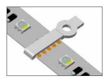
2. After fixing, determine the position of the light strip to install the fixed card holder (the position of the light strip bead and the light strip or the position of the light strip pad)
