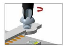
4. Align the screws with the round hole fixing the card seat and turn clockwise to ensure that the screws have locked the card seat. (Please use special tools for screws)
